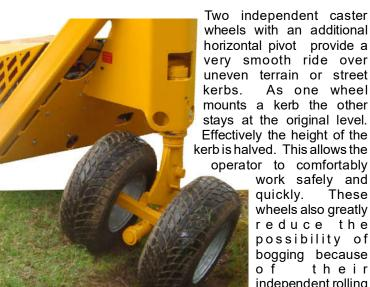
Two independent caster wheels with an additional horizontal pivot provide a very smooth ride over uneven terrain or street As one wheel mounts a kerb the other stays at the original level. Effectively the height of the kerb is halved. This allows the
